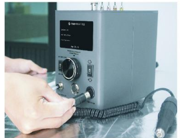
STEP 4 Connect the Micro motor at the front right side.
