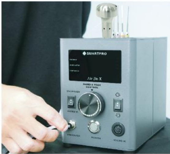
STEP 3 Connect the Engraver Handpiece at the front-left side.
