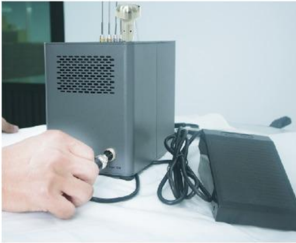
STEP 1 Connect Foot pedal at the back-Right side.
